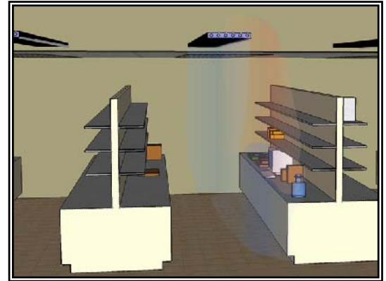
Figure XV: Proposed Chilled Beam Application in Lab
